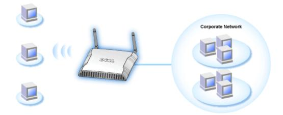
• Wireless repeater: In this mode the Access Point is able to extend the wireless range of a root Access Point that is on the corporate network to remote wireless computers.
