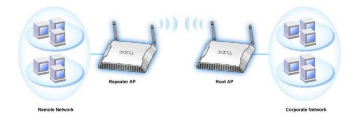
The Dell Wireless 4350 Small Network Access Point supports up to 64 wireless clients. It runs at speeds up to 54 **Megabits per second** (Mbps), and the LAN (wired) port runs at 10/100 Mbps. The maximum distance between the Access Point and each Wireless computer is 300 feet. This distance may be less depending on your environment.
